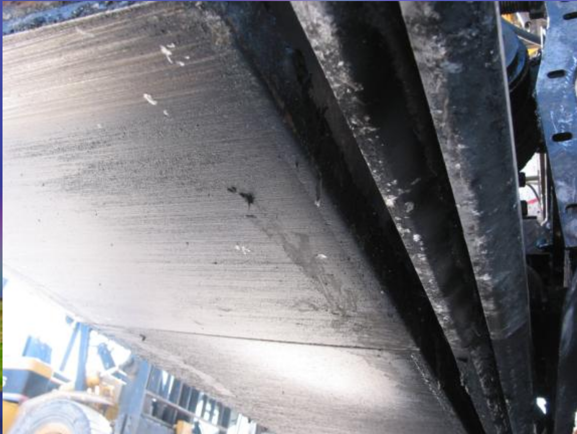
Tamping bars on heavy, tamping bar, vibratory screed paver
